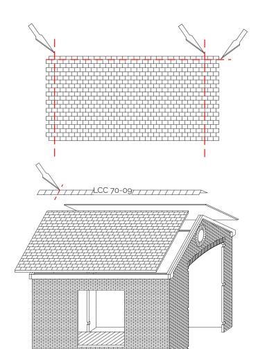
Trim the roof panels LCC 70-13DW to size. They should end up approximately 164mm wide and 88mm high. Make sure to cut them oversized at first and then fit to exact size. Roof panels should be resting with the edge touching the facia boards and the ends should be flush with the barge boards.
