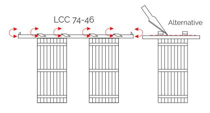
Assemble the sliding gates by first folding the tab on the ends of the rail (only use one rail from the fret for this kit). Glue the rail to the sliding gates and then fold the tabs over to form a hinge. Alternatively after gluing the rail to the gates cut the tabs off from the gates for easier and alternative look.
