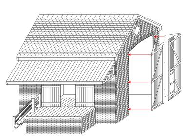
Fold the train gates LCC 74-02 and LCC 74-03 in half with some watered down glue between. Make sure to align them neatly and press them for a few minutes between something heavy so they bond well and are flat.
