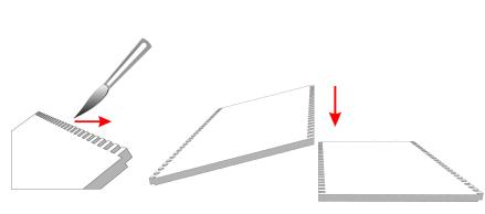
Recommended way of gluing parts together is to apply PVA glue to the interlocking bricks working from back of the part to the front.
