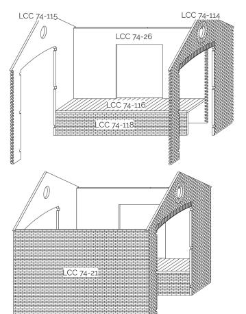
Start by joining LCC 74-26 with LCC 74-114 and LCC 74-115. Make sure to glue in the gate panels as shown on the diagram. The wider parts should be facing the loading door. Fit the inner platform which will stabilise the construction.
