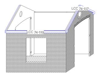
Glue the barge boards LCC 74-117 to the gate panels making sure they are well aligned with the slopes of the gable.
